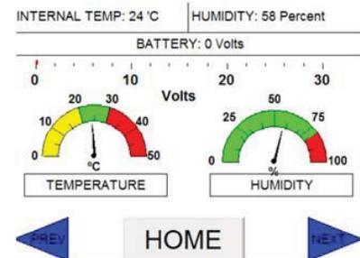
The control system is self contained and has built in power redundancy for 24 hours, independent of any additional UPS system.
